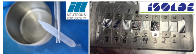
Figure 1: Left: Enclosed stable Xe sample ready for neutron capture at ILL. Right: metal matrix used for Xe implantation at the GLM beamline.
