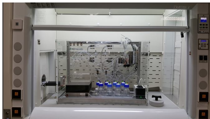
Figure 3: Automatic radiochemistry set-up
