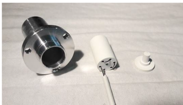
Figure 6: Heater assembly for reactants with low boiling point (first prototype). From left to right: Aluminum case, heating cartridge: boron nitride insulating the tantalum heating wires and contains the sulfur powder, plug.
