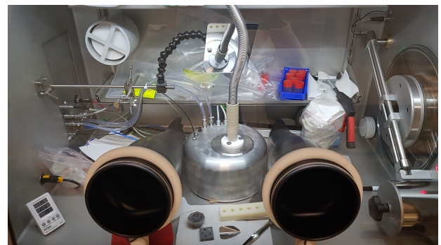
Figure 12: Inert atmosphere nuclear glovebox for the handling and the thermal analysis of UC x sample under controlled atmosphere.
