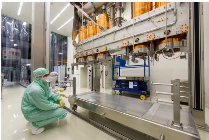
Fig. 1: Assembly of the first HIE-ISOLDE cryomodule, with its five copper cavities in the new SM18 cleanroom ( http://cds.cern.ch/record/2007275 ).
