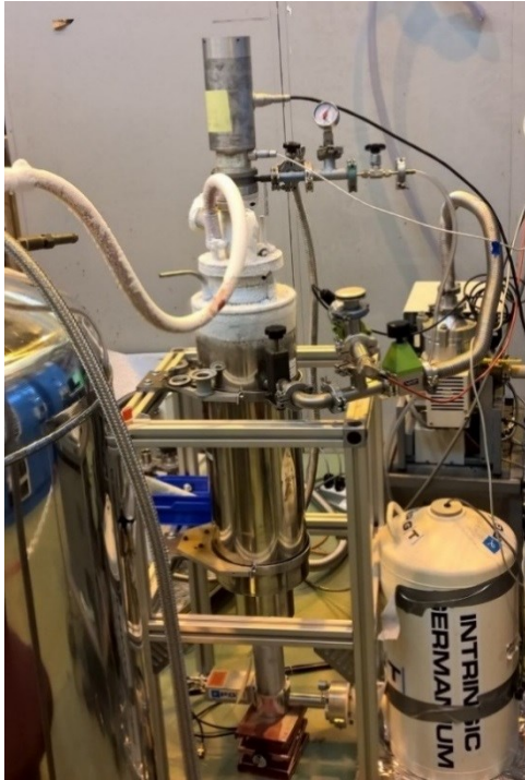
Fig. 2: The IKS cryostat during testing. The Mössbauer drive system is on top of the cryostat, and the detector below.
