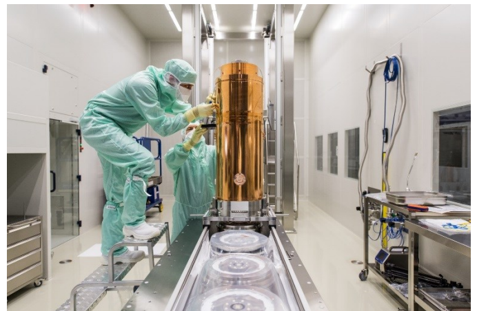
Fig. 7: Installation of instrumentation on the rinsed superconductive cavity before assembly into CM1.
