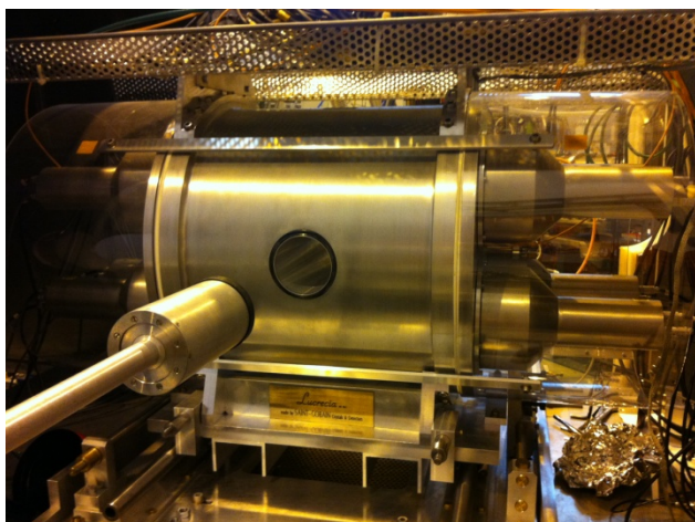
Fig. 1: Picture of the "Lucrecia" Total Absorption Spectrometer located in the ISOLDE hall and used in the IS370 experiment for the study of the ^{72}\text{Kr} beta decay described in this article.
