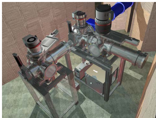
Fig.1: CAD drawing of both chambers in the GLM cave. The schematic blue structure in the back is a dummy of the ISOLDE beam line. The big chamber on the right side is the new implantation chamber while the smaller chamber on the left side is the deceleration chamber. At the exit of the deceleration chamber the valve on the left providing the possibility of shooting through both chambers and adding additional chambers is also visible.
